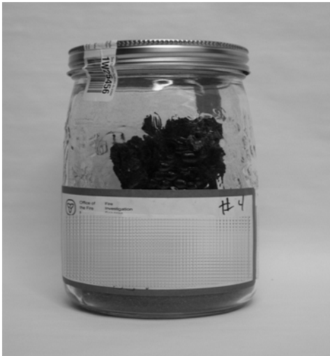
Figure 3: Glass Mason jar with fire debris.
